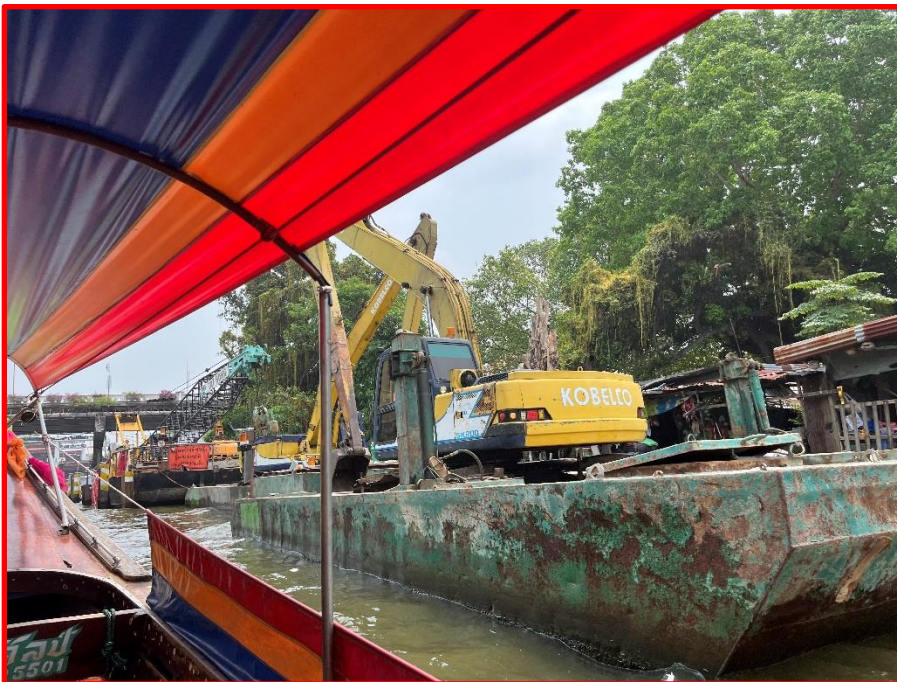
One of many long stick excavators on a barge.
